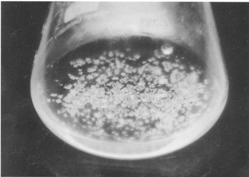
Fig. 3. Starlike crystals growing in the liquid phase of sample 3 at 33^\circ\text{C} . Initial concentrations: 67.3 wt% LiBr, 7.65 wt% \text{NH}_3 , and 25.05 wt% \text{H}_2\text{O} .
