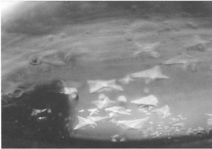
Fig. 2. The first primary crystallites appearing in the liquid phase of sample 3 at 43^\circ\text{C} . Concentrations: 67.3 wt% LiBr, 7.65 wt% \text{NH}_3 , and 25.05 wt% \text{H}_2\text{O} .
